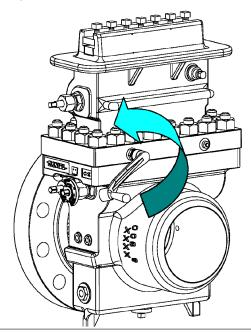
2. Wait several seconds while the pressure in the Top (14) equalizes to that of the Body (4).
