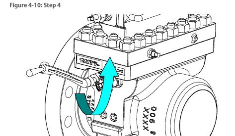
5. Continue to rotate the Lower Plate Carrier Shaft (6) located on the Body (4) until the Upper Plate Carrier Shaft (7) located in the Top (14) begins to rotate
