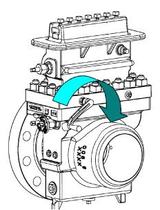
9. Using the Operating Wrench (2) rotate the Slide Valve Shaft (5) until it stops and the CLOSED position specified on the Indicator Plate (5A) is in line with the Indicator Pointer (5B).
