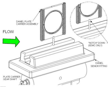
Figure 3-2: Orientation of plate carrier (8DM or 8DMC) prior to installation
