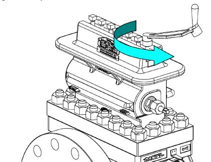
15. Once the Clamping Bar Screws (11) are loose, rotate the Upper Plate Carrier Shaft (7) located in the Top (14) with the Operating Wrench (2), until the Plate Carrier (8DM or 8DMC) taps against the Sealing Bar (9 or 9HP) freeing it from the Top (14).
