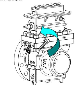
40. Wait several seconds for the Top (14) to reach pressure equilibrium with the line pressure contained in the Body (4).
