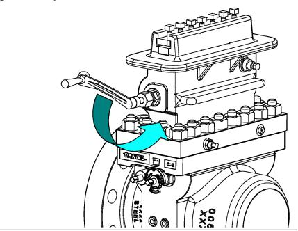
30. Slide the Clamping Bar (12 or 12HP) containing the Clamping Bar Screws (11), the Sealing Bar (9) from the Top (14).
