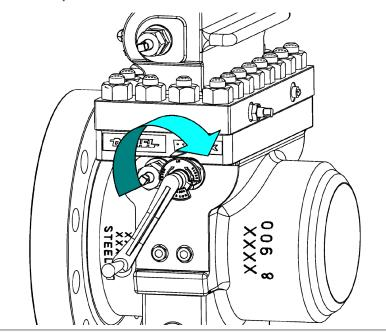
42. Rotate the Upper Plate Carrier Shaft (7) located in the Top (14) with the Operating Wrench (2) in the direction to lower the Orifice Plate Carrier (8DM or 8DMC) into the Body (4).
