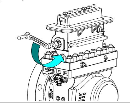
8. Close the Equalizer Valve (1) with the Operating Wrench (2).
