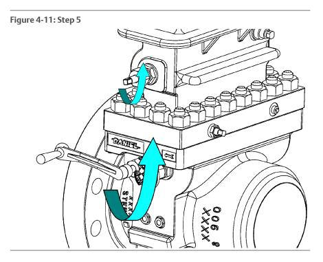
6. Move the Operating Wrench (2) from the Lower Plate Carrier Shaft (6) located in the Body (4) on the Upper Plate Carrier Shaft (7) located in the Top (14).
