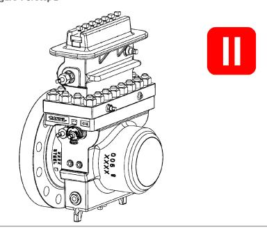
3. Using the Operating Wrench (2) rotate the Slide Valve Shaft (5) until it stops and the OPEN position specified on the Indicator Plate (5A) is in line with the Indicator Pointer (5B).
