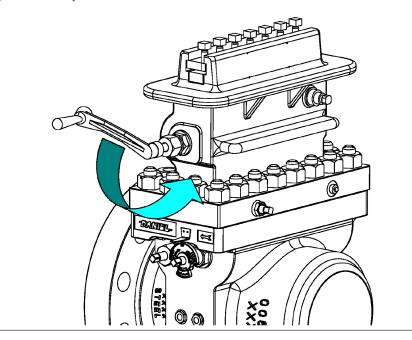
16. Slide the Clamping Bar (12 or 12HP) containing the Clamping Bar Screws (11), the Sealing Bar (9 or 9HP) from the Top (14).
