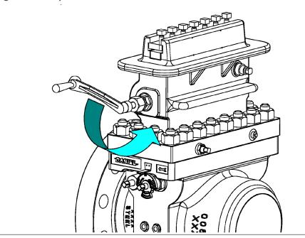
16. Slide the Clamping Bar (12 or 12HP) containing the Clamping Bar Screws (11), the Sealing Bar (9 or 9HP) from the Top (14).
