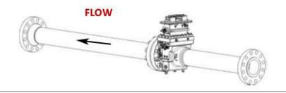
Figure 2-7: Parallel to the ground "Left side" position
