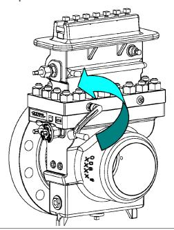
28. Wait several seconds for the Top (14) to reach pressure equilibrium with the line pressure contained in the Body (4).
