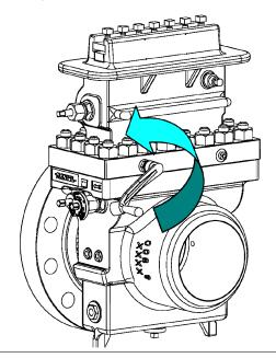
2. Wait several seconds while the pressure in the Top (14) equalizes to that of the Body (4).
