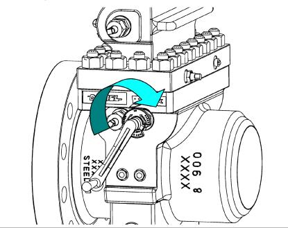
30. Rotate the Upper Plate Carrier Shaft (7) with the Operating Wrench (2) in the direction to lower the Orifice Plate Carrier (8DM or 8DMC) into the Body (4).
