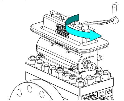
29. Once the Clamping Bar Screws (11) are loose, it may be necessary to use the Operating Wrench (2) to tap against the Sealing Bar (9 or 9HP) freeing it from the Top (14).
