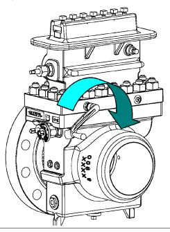
9. Using the Operating Wrench (2) rotate the Slide Valve Shaft (5) until it stops and the CLOSED position specified on the Indicator Plate (5A) is in line with the Indicator Pointer (5B).
