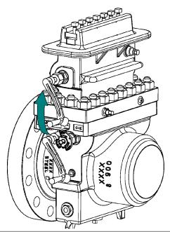
7. Rotate the Upper Plate Carrier Shaft (7) located in the Top (14) until the Plate Carrier (8DM or 8DMC) stops against the Sealing Bar (9 or 9HP).
