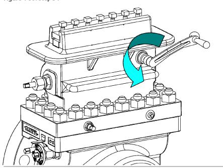
Steps 35 and 36 are ONLY required for Seniors equipped with grease assisted, metal-to-metal slide valves. Personnel operating the Daniel Senior Orifice Fittings equipped with O-Ring seal "soft seat" design slide valves skip to step 37.
