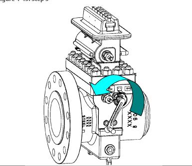
10. Open the Bleeder Valve (10B) with the Operating Wrench (2).
