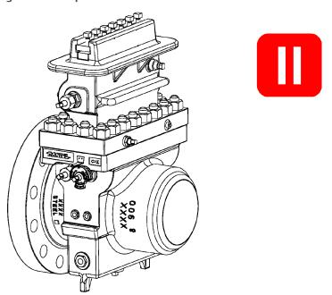
3. Using the Operating Wrench (2) rotate the Slide Valve Shaft (5) until it stops and the OPEN position is specified on the Indicator Plate (5A) with the Indicator Pointer (5B).
