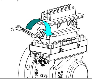
31. Rotate the Lower Plate Carrier Shaft (6) with the Operating Wrench (2) until the Orifice Plate Carrier (8DM or 8DMC) cannot be lowered further.
