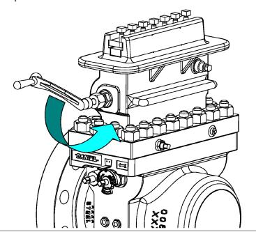
8. Close the Equalizer Valve (1) with the Operating Wrench (2).
