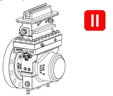
29. Using the Operating Wrench (2), rotate the Slide Valve Shaft (5) to the OPEN position.
