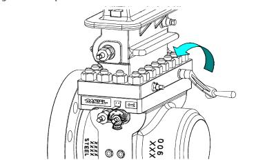
26. Return the stem to the Grease Gun (23) and begin turning it clockwise by hand into the Grease Gun (23) until resistance is felt. Once this is done, use the supplied Operating Wrench (2) to continue to turn the stem at a rate of 4 to 6 turns per minute.
