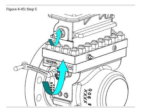
6. Move the Operating Wrench (2) from the Lower Plate Carrier Shaft (6) located in the Body (4) on the Upper Plate Carrier Shaft (7) located in the Top (14).
