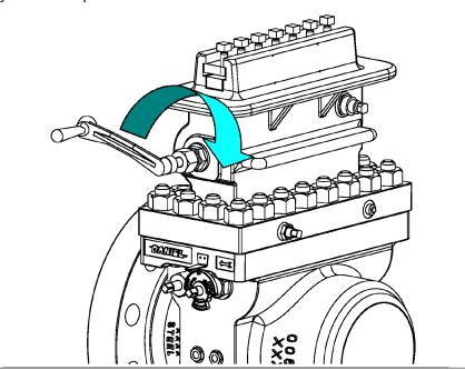
43. Rotate the Lower Plate Carrier Shaft (6) with the Operating Wrench (2) until the Orifice Plate Carrier (8DM or 8DMC) cannot be lowered further.
