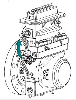
7. Rotate the Upper Plate Carrier Shaft (7) located in the Top (14) until the Plate Carrier (8DM or 8DMC) stops against the Sealing Bar (9, 9HP).
