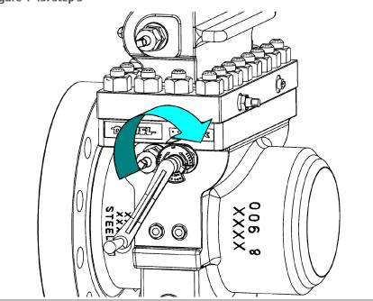
4. Rotate the Lower Plate Carrier Shaft (6), located on the Body (4), using the Operating Wrench (2) in a direction that will move the Plate Carrier (8DM or 8DMC) out of the Body (4) into the Top (14).
