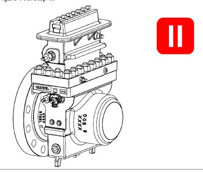
41. Using the Operating Wrench (2), rotate the Slide Valve Shaft (5) to the OPEN position.
