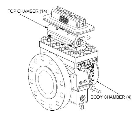
Therefore, using a Senior may eliminate the need for bypass piping, valves, and other fittings necessary with conventional orifice fitting installations. Maintenance technicians can replace and repair all parts of the Senior, including the slide valve assembly, without removing the Body (4) from the line (refer to Maintain).
