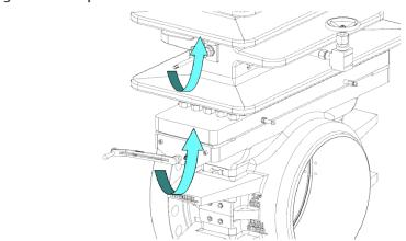
6. Move the Operating Wrench (2) from the Lower Plate Carrier Shaft (6) located in the Body (4) on the Upper Plate Carrier Shaft (7) located in the Top (14).
