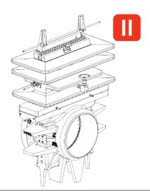
41. Using the Operating Wrench (2), rotate the Slide Valve Shaft (5) to the OPEN position.
