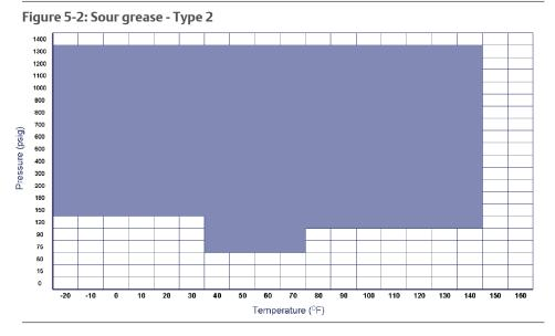
Pressure (psig) v. Temperature (°F) SOUR GAS GREASE - TYPE 2 - Part Number: 1-213-04-102 OPTIMUM SEALING RANGE WITH NITROGEN FOR A 3" ANSI 600 SENIOR FITTING UNDER LABORATORY CONDITIONS. Colored coordinate boxes indicate no detectable leakage at that Temperature and Pressure for 30 minutes.
