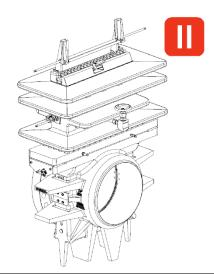
3. Using the Operating Wrench (2) rotate the Slide Valve Shaft (5) until it stops and the OPEN position is specified on the Indicator Plate (5A) with the Indicator Pointer (5B).
