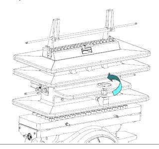
Step 47 and 48 are ONLY required for Seniors equipped with grease assisted, metal-to-metal slide valves. Personnel operating the Daniel Senior Orifice Fitting equipped with O-Ring seal "soft seat" design slide valves skip to step 49.
