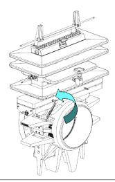
2. Wait several seconds while the pressure in the Top (14) equalizes to that of the Body (4).
