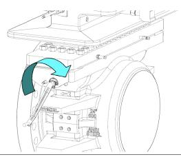
4. Rotate the Lower Plate Carrier Shaft (6), located on the Body (4), using the Operating Wrench (2) in a direction that will move the Plate Carrier (8DM or 8DMC) out of the Body (4) into the Top (14).
