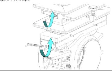
6. Move the Operating Wrench (2) from the Lower Plate Carrier Shaft (6) located in the Body (4) on the Upper Plate Carrier Shaft (7) located in the Top (14).
