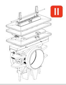
3. Using the Operating Wrench (2) rotate the Slide Valve Shaft (5) until it stops and the OPEN position specified on the Indicator Plate (5A) is in line with the Indicator Pointer (5B).
