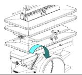
9. Using the Operating Wrench (2) rotate the Slide Valve Shaft (5) until it stops and the CLOSED position specified on the Indicator Plate (5A) is in line with the Indicator Pointer (5B).
