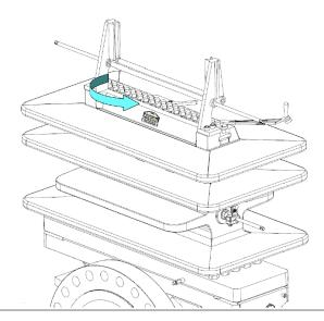
15. Once the Clamping Bar Screws (11) are loose, rotate the Upper Plate Carrier Shaft (7) located in the Top (14) with the Operating Wrench (2), until the Plate Carrier (8DM or 8DMC) taps against the Sealing Bar (9 or 9HP) freeing it from the Top (14).
