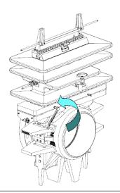
28. Wait several seconds for the Top (14) to reach pressure equilibrium with the line pressure contained in the Body (4).
