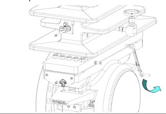
26. Return the stem to the Grease Gun (23) and begin turning it clockwise by hand into the Grease Gun (23) until resistance is felt. Once this is done, use the supplied Operating Wrench (2) to continue to turn the stem at a rate of 4 to 6 turns per minute.
