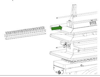
22. Tighten each Clamping Bar Screw (11) located on the Clamping Bar (12) to the torque recommended in this manual (refer to Torque information).
