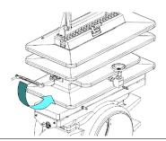
8. Close the Equalizer Valve (1) with the Operating Wrench (2).
