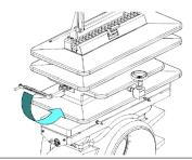
16. Slide the Clamping Bar (12) containing the Clamping Bar Screws (11), the Sealing Bar (9 or 9HP) from the Top (14).
