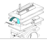
43. Rotate the Lower Plate Carrier Shaft (6) with the Operating Wrench (2) until the Orifice Plate Carrier (8DM) cannot be lowered further.
