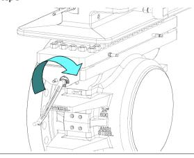
4. Rotate the Lower Plate Carrier Shaft (6) located on the Body (4) using the Operating Wrench (2) in a direction that will move the Plate Carrier (8DM) out of the Body (4) into the Top (14).
