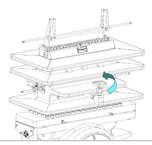
Steps 11 and 12 are ONLY required for the Seniors equipped with grease assisted, metal-tometal slide valves. Personnel operating the Senior equipped with O-Ring seal "soft seat" design slide valves skip to step 13.
