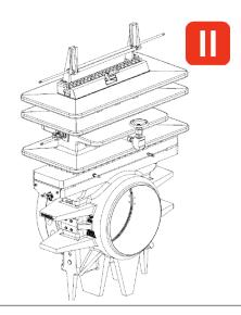
29. Using the Operating Wrench (2), rotate the Slide Valve Shaft (5) to the OPEN position.
