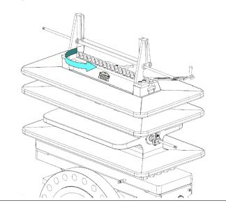
29. Once the Clamping Bar Screws (11) are loose, it may be necessary to use the Operating Wrench (2) to tap against the Sealing Bar (9) freeing it from the Top (14).
