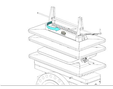
15. Once the Clamping Bar Screws (11) are loose, rotate the Upper Plate Carrier Shaft (7) located in the Top (14) with the Operating Wrench (2), until the Plate Carrier (8DM) taps against the Sealing Bar (9) freeing it from the Top (14).
