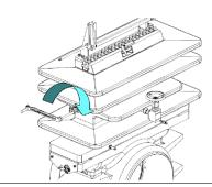
31. Rotate the Lower Plate Carrier Shaft (6) with the Operating Wrench (2) until the Orifice Plate Carrier (8DM) cannot be lowered further.
