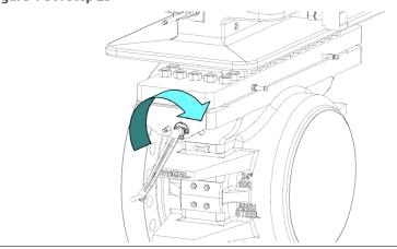
30. Rotate the Upper Plate Carrier Shaft (7) with the Operating Wrench (2) in the direction to lower the Orifice Plate Carrier (8DM) into the Body (4).
