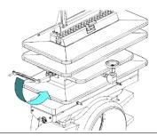
16. Slide the Clamping Bar (12 or 12HP) containing the Clamping Bar Screws (11), the Sealing Bar (9 or 9HP) from the Top (14).
