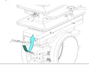
5. Continue to rotate the Lower Plate Carrier Shaft (6) located on the Body (4) until the Upper Plate Carrier Shaft (7) located in the Top (14) begins to rotate
