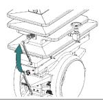
7. Rotate the Upper Plate Carrier Shaft (7) located in the Top (14) until the Plate Carrier (8DM) stops against the Sealing Bar (9).
