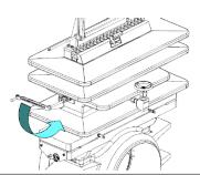
30. Slide the Clamping Bar (12) containing the Clamping Bar Screws (11), the Sealing Bar (9) from the Top (14).
