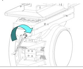
42. Rotate the Upper Plate Carrier Shaft (7) located in the Top (14) with the Operating Wrench (2) in the direction to lower the Orifice Plate Carrier (8DM) into the Body (4).
