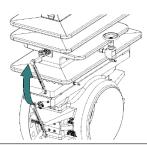
7. Rotate the Upper Plate Carrier Shaft (7) located in the Top (14) until the Plate Carrier (8DM or 8DMC) stops against the Sealing Bar (9, 9HP).
