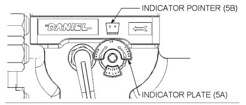
Prior to performing any maintenance or Orifice Plate (13) installation and removal operations on the Senior, personnel must visually confirm the presence of the indicator Plate (5A) on the Slide Valve Shaft (5) and the Indicator Pointer (5B) on the Body (4). Both the indicator plate and the indicator pointer must be installed to operate this equipment safely.
