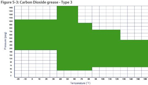
Pressure (psig) v. Temperature (°F) CARBON DIOXIDE GREASE - TYPE 3 - Part Number: 1-213-04-101 OPTIMUM SEALING RANGE WITH NITROGEN FOR A 3" ANSI 600 SENIOR FITTING UNDER LABORATORY CONDITIONS. Colored coordinate boxes indicate no detectable leakage at that Temperature and Pressure for 30 minutes.
