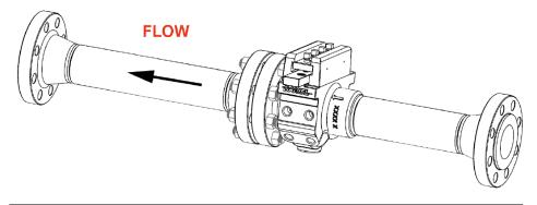
Figure 2-5: Horizontal flow - "left side" position (parallel to the ground)
