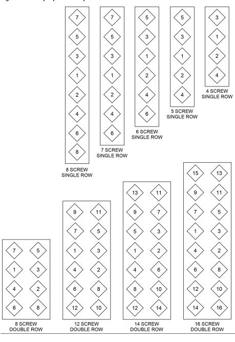
Figure 5-1: Torque pattern sequences
