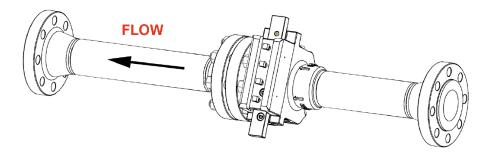
Installing the fitting in a vertical flow direction gives a product owner and operating personnel the option to fix the fitting in any position parallel to the ground. Although the insertion of the fitting in the vertical flow direction can be vertical UP or vertical DOWN, it is recommended the fitting be in the vertical down flow direction to reduce the potential of debris collecting on the orifice plate.
